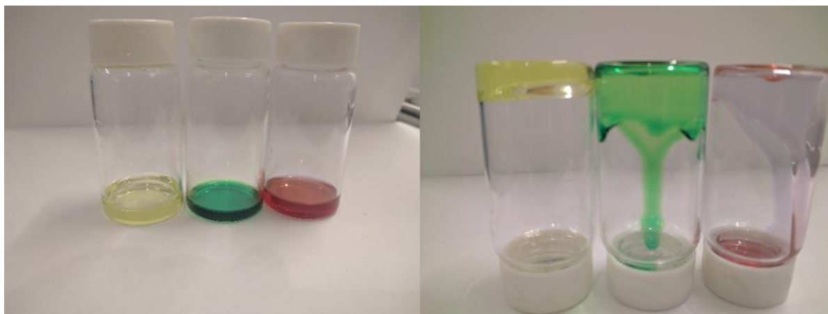
Figure 2.2. [\text{P}_{66614}^+]_2[\text{MnCl}_4^{2-}] (left), [\text{P}_{66614}^+][\text{Ni(II)(hfacac)}_3^-] (middle), and [\text{P}_{66614}^+][\text{Nd(III)(hfacac)}_4^-] (right) before and after inversion for 1 second.
